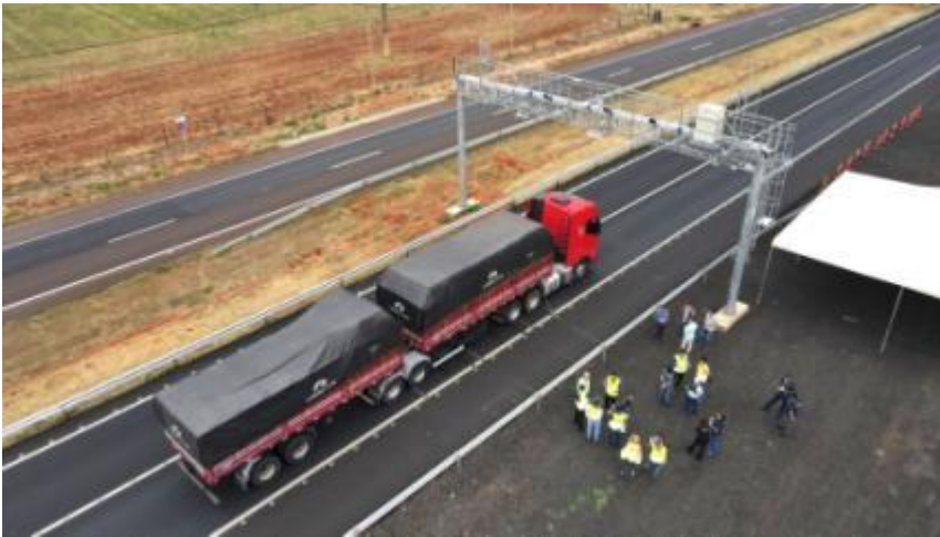
Kistler's system for electronic tolling with Weigh In Motion
