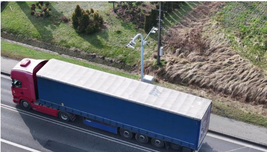
APM's WIM Prosystem with DSRC antenna
