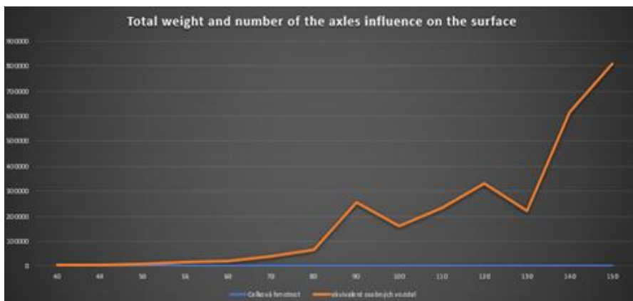
Effects of traffic loading on road lifespan.
