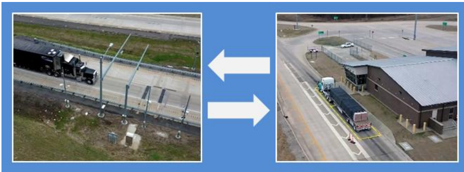
Referencing static scale data is one way to reduce drift
