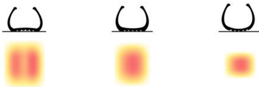
Footprint of under- (left), correctly (center), and over-inflated (right) tires
