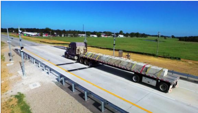
A test truck crosses the WIM scales at the U.S. 412 VWS site
