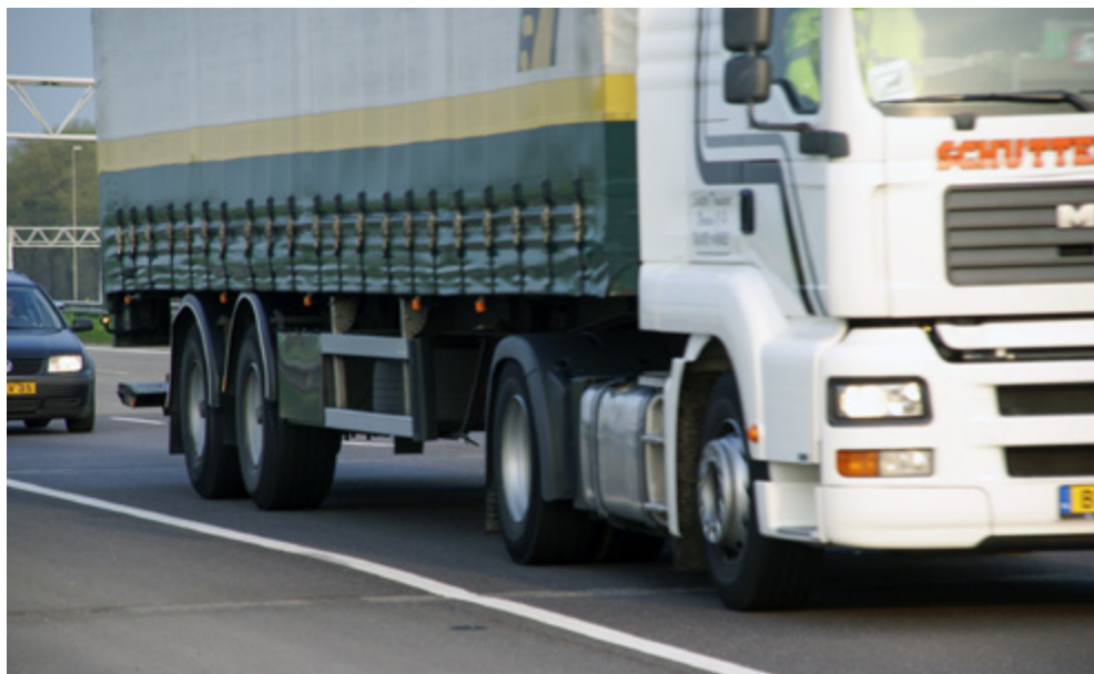
Figure 6.1: A 4-axle calibration truck passing WIM sensors
