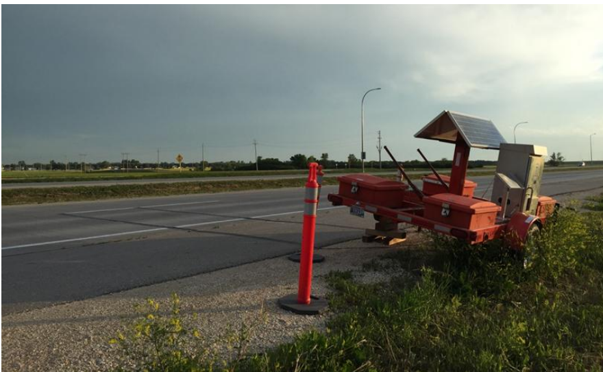
Portable WIM system Installed in Manitoba, Canada
