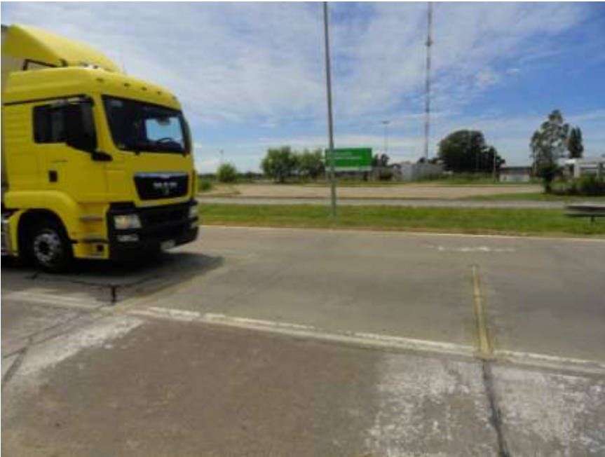
Intercomp OIML R134 certified 2 sensor row WIM system.
