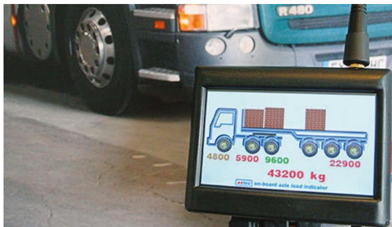
Figure 3.8: Display of On-Board Weighing measurements
