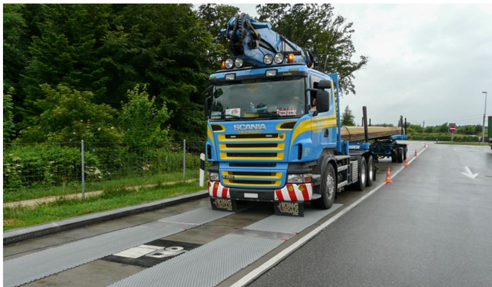
Figure 4.8: Road side weight enforcement using static scales in Switzerland
