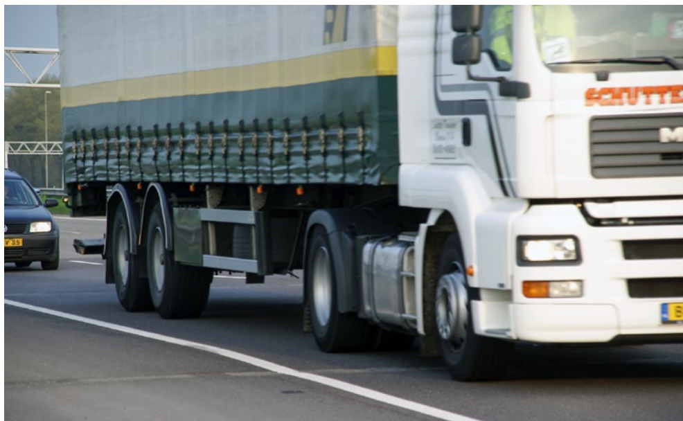
Figure 6.1: A 4-axle calibration truck passing WIM sensors
