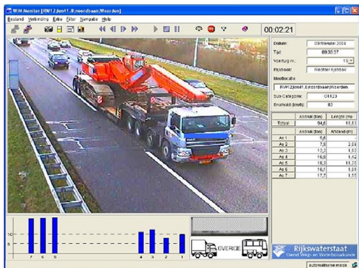
Figure 3.2: Example of data measured by an extended WIM system. Source: RIJKSWATERSTAAT
